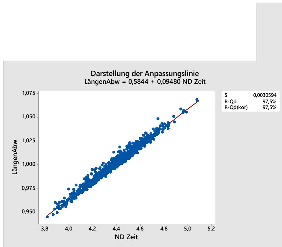
Deviation of Length =  $f$  (pressure time; tool temperature)
