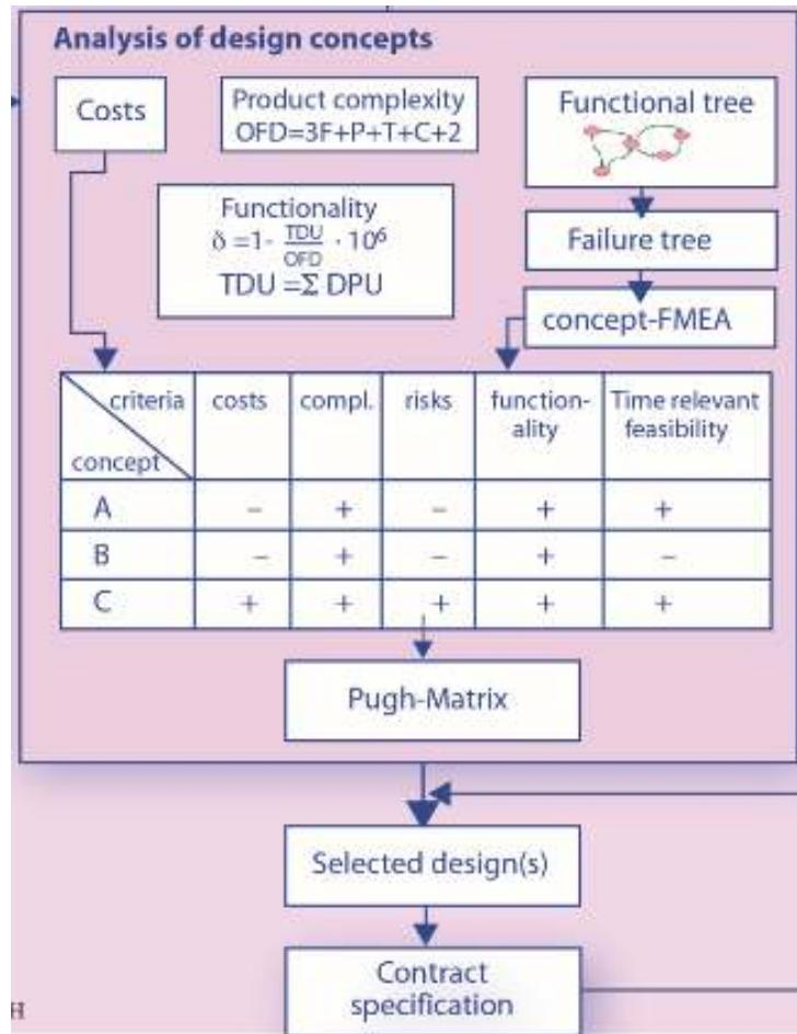
As well FMEA – Failure Mode and Effect Analysis - as FTA – Fault Tree Analysis will be attended.
